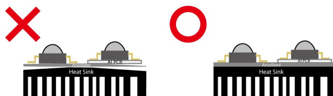
<Figure 19 Edixeon ® ARC series assemble with heatsink>
